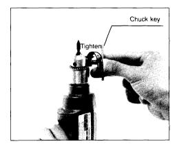
After use, return the chuck key to the storage cavity on the tool.
